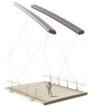
FIGURE 2 — CONCEPTUAL ISOMETRIC CROSS-SECTION OF ARCH RIBS AND DECK (IMAGE COURTESY OF RFR)
